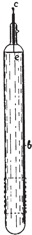
Figure 2. Drawing illustrates Tesla’s unipolar vacuum tube, consisting of a glass bulb ( b ), a single electrode ( e ), and a lead-in conductor ( c ). The tube can be adapted for use with two electrodes by placing the second electrode at the levels indicated by the dotted lines. Published in Electrical Review, New York , April 1, 1896. (Reprinted from reference 3.)
